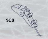
Type **SCB** are consist of galvanised steel aircraft cables sized to resist seismic loads with a minimum safety factor of two and arranged to provide all-directional restraint. It has a hole for anchoring to equipment or structure.
